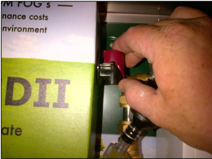
Step 5: Remove maroon cover from the top of the Bag in Box tap and remove white tag from the bottom of the tap
